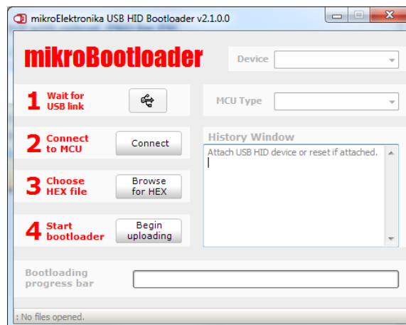
Figure 6. Programmer Software in MikroC Pro for PIC.
